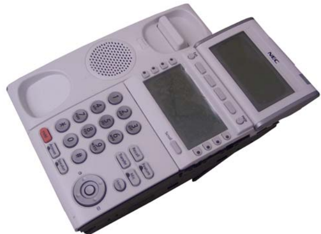
Figure 5-93 8LKD (LD)-L UNIT Installed
