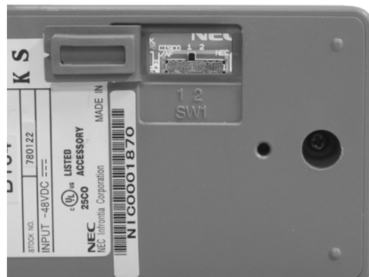
Figure 6-21 In-Line Power Adapter Switch Settings
