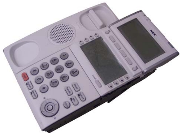
Figure 5-99 8LKI (LD)-L UNIT Installed
