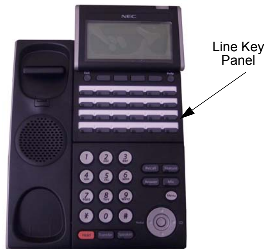
Figure 5-48 Installing the Line Key Panel
